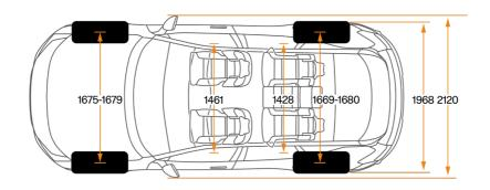
Dimensions (mm): L-4900 mm H-1614 mm W-2120 mm
