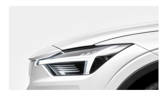
Headlights Polestar 2's LED headlights combine energy efficiency with an intricate design. They automatically adjust in intensity depending on the ambient light to create optimal illumination in all conditions.
