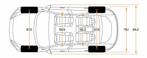
Dimensions (inches): L-190.7" H-60.4" W-84.2" Wheelbase (inches): 118.1" Tyre specs: 21" 265/45 295/40 – 22" 265/40 295/35 Luggage volumes front/rear (cubic feet): 0.5 cubic feet / 18.9 cubic feet
